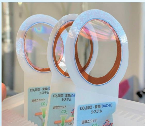
Photo of the large and free-standing nanomembranes – membrane with a thickness of a few hundred nanometers and a diameter of several centimeters (aspect ratio of ~10 6 )
