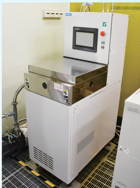
Parallel plate RIE system "RIE-10NR" in the cleanroom
