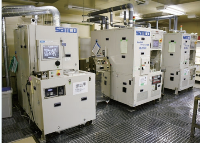
From left: First unit of Bosch process-compatible silicon deep etching system “RIE-800iPB” Chlorine gas-based ICP etching system “RIE-101iPH” Fluorine gas-based ICP etching system “RIE-101iPH”
