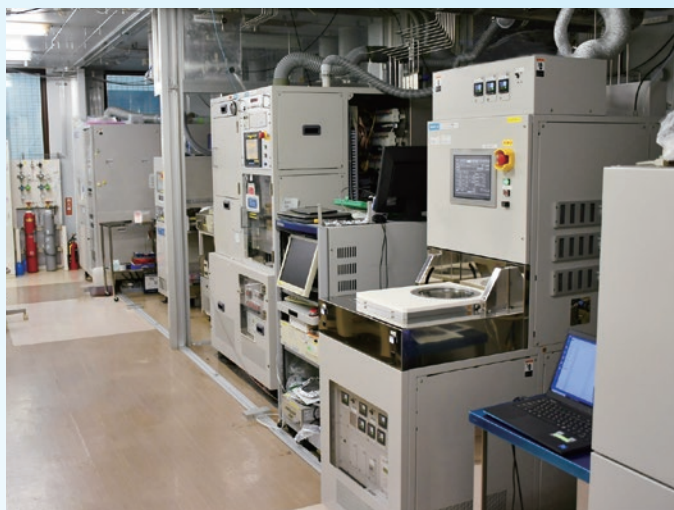
Anode/cathode switching plasma CVD system 'PD-200STL'. ICP etching system 'RIE-10iPH' Parallel plate dry etching systems 'RIE-10NR', 'RIE-10NRN' Liquid source CVD system 'PD-100ST'.
