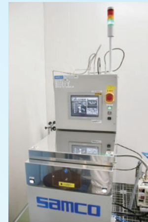
Parallel-plate RIE system "RIE-10NR," introduced in 2026.
